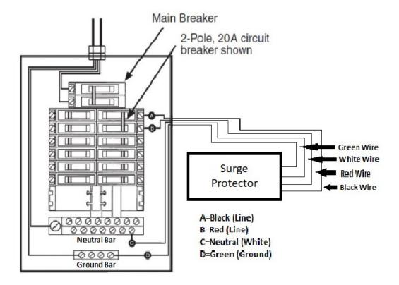
Install as close to the main breaker as possible. It is recommended per most building codes to connect to a 20A double pole circuit breaker.
